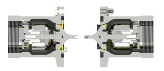
When ERC activates and separates it allows the halves to close instantly thus ensuring leak proof spilling on both halves
